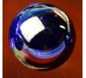
Fusion fuel is encased in a sphere of high density carbon (synthetic diamond) the size of a pepper corn
