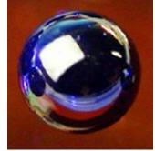
Fusion fuel is encased in a sphere of high density carbon (synthetic diamond) the size of a pepper corn
